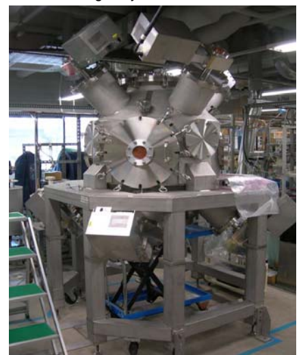
Fig.2 Microwave furnace for ironmaking, which allows the raw materials to be irradiated by directional microwave.
